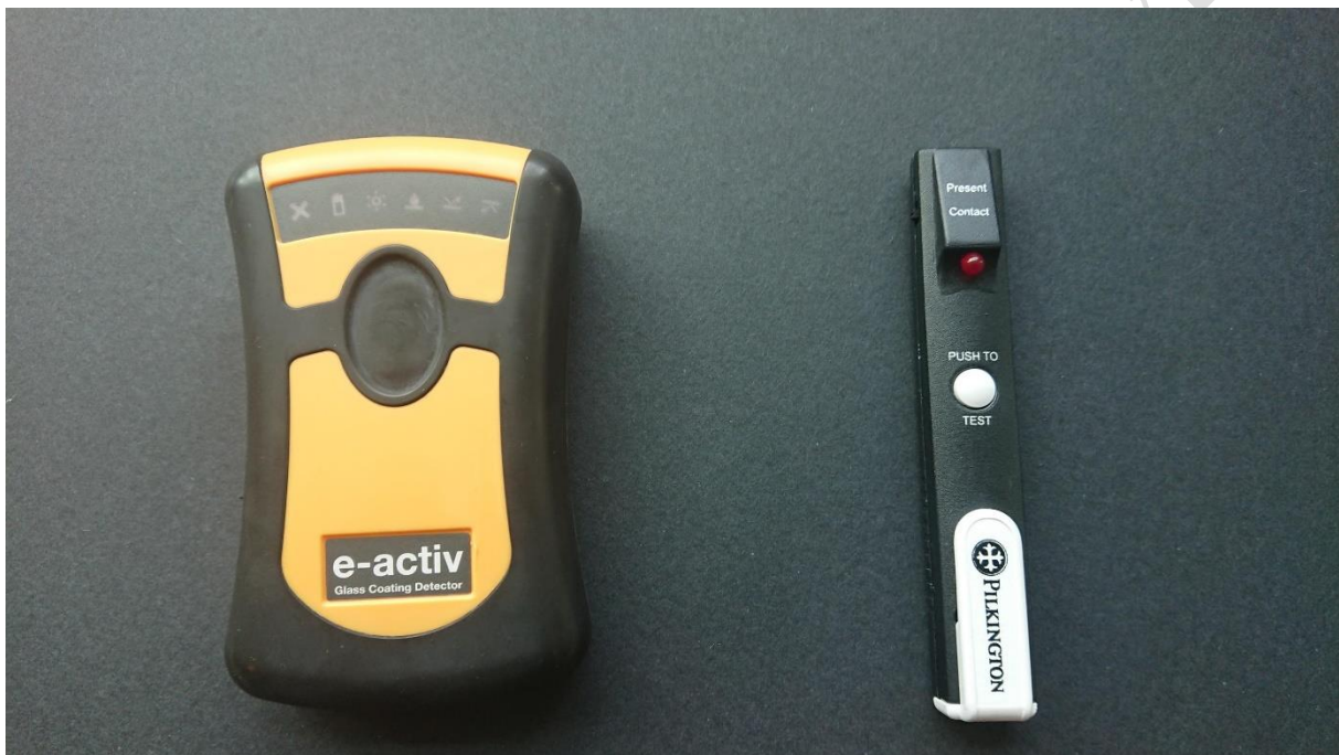
Figure 2: Examples of low-e coating detectors
